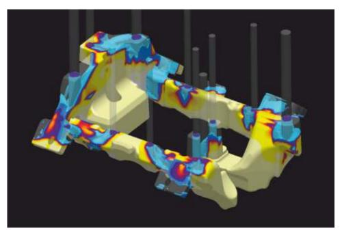
During the engineering phase, a simulation on core heating / shooting / curing + pouring can be performed using Magmasoft software; it allows to get rapidly to the definition of the final casting compliant to the customer metallurgical standards.
