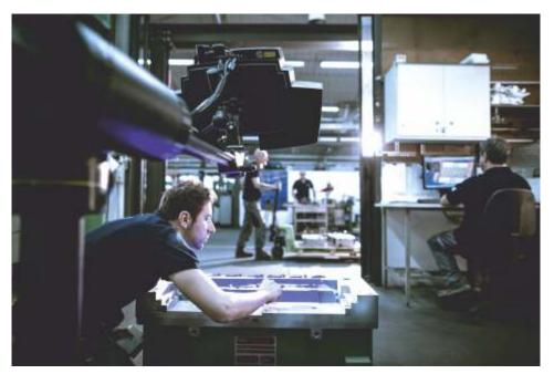
Through ATOS GOM and METROLOG software, the measuring machines compare the 3D model to the manufactured tooling, displaying any tolerance deviation, if any. Dimensional tests are performed during the whole production process. Along with the tooling, the customer is provided with the complete 3D engineering data, related 2D drawings sets and the dimensional inspection reports. This documentation facilitates customer tasks related to product management and especially to maintenance.
